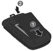
Note: The battery must be properly installed before charging the battery or switching on the phone.
